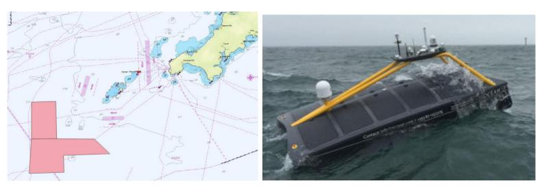
There may be up to 4 USVs in operation at any one time and each is piloted remotely 24hrs a day. Each USV is 4.5m long, 2.2m wide and will travel at approximately 3.5kts. When the USVs are being launched they will be escorted by a support vessel which will operate from the harbour to the Spencer's Ledge buoy and vice versa for recovery. Each USV is fitted with AIS, navigational lights and sound signals, active radar reflector and the superstructure painted yellow (see above image).
